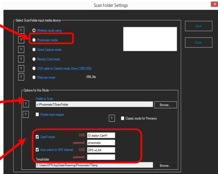
The CamFi controller will generate a network to which the ID station will connect. This network has a certain name (SSID) and password. Every CamFi controller we ship along with ID station generates a network called "ID station Camfi" and requires a password "photomatic".
